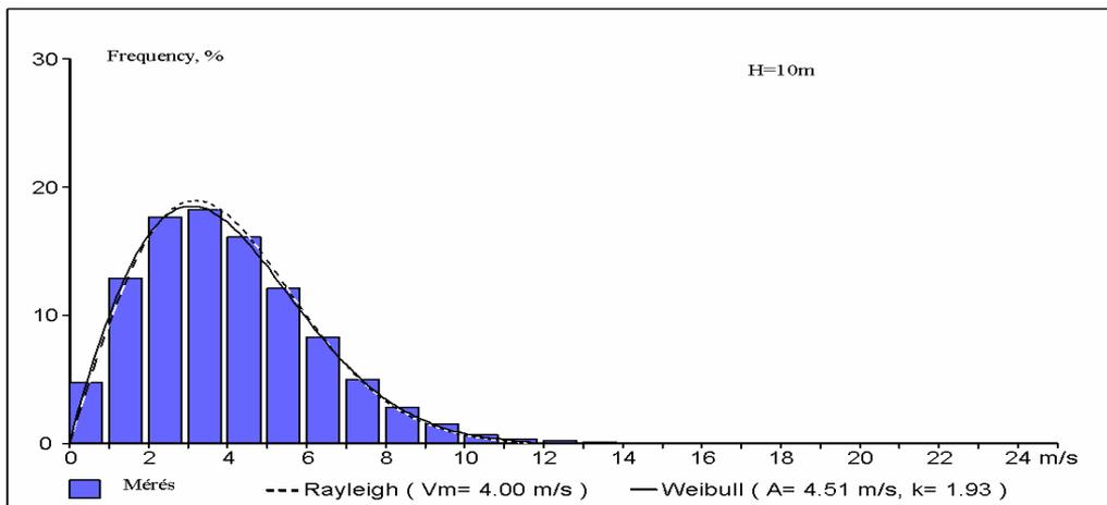
Fig. 3.1. Wind speed distribution at 10 m height
