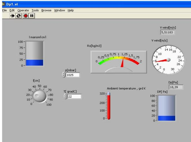
Fig. 3.5. Wind speed measurements, Lab View Model
