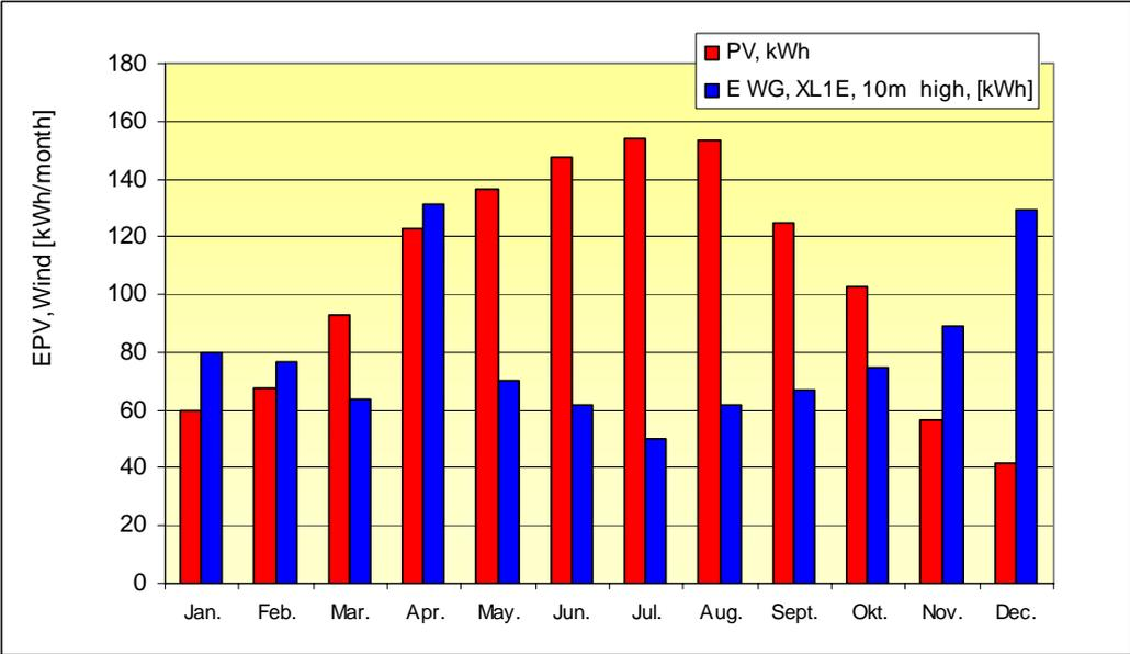
Fig. 3.12. The monthly average energy production of 1 kW<sub>p</sub> power PV and Wind hybrid system
