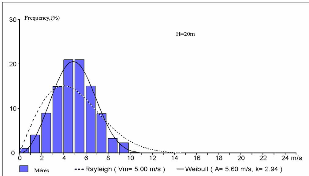
Fig. 3.2. The wind speed distribution at 20 m height
