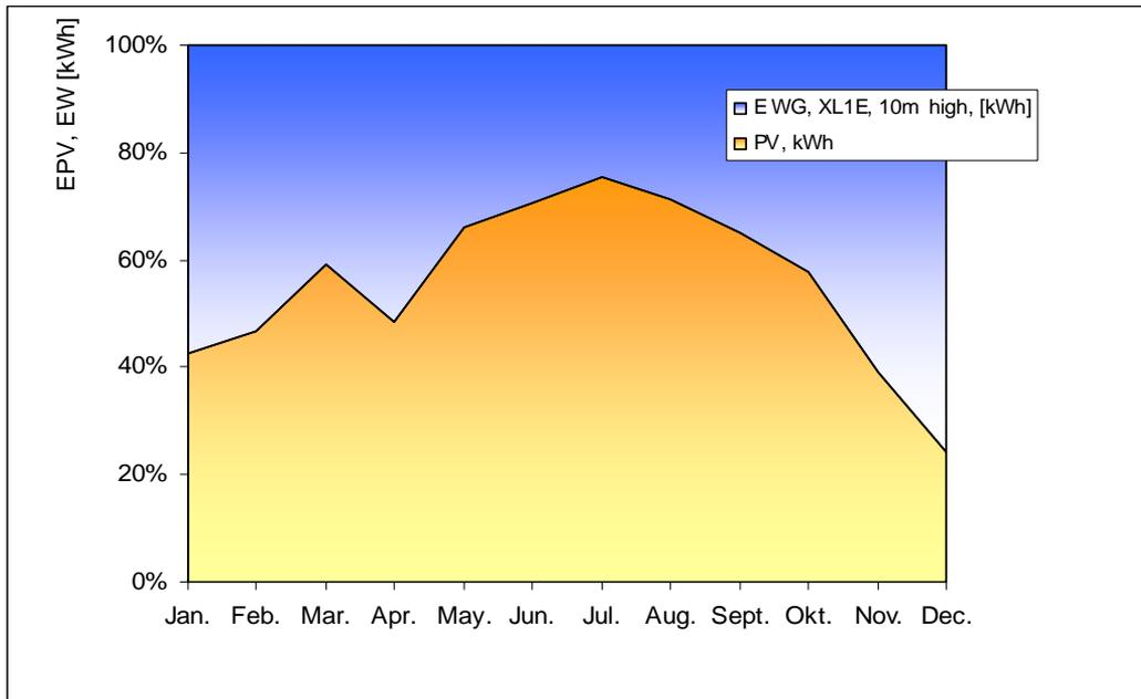
Fig. 3.13. The monthly average energy production of 1 kW<sub>p</sub> PV 1 kW<sub>p</sub> Wind energy hybrid system
