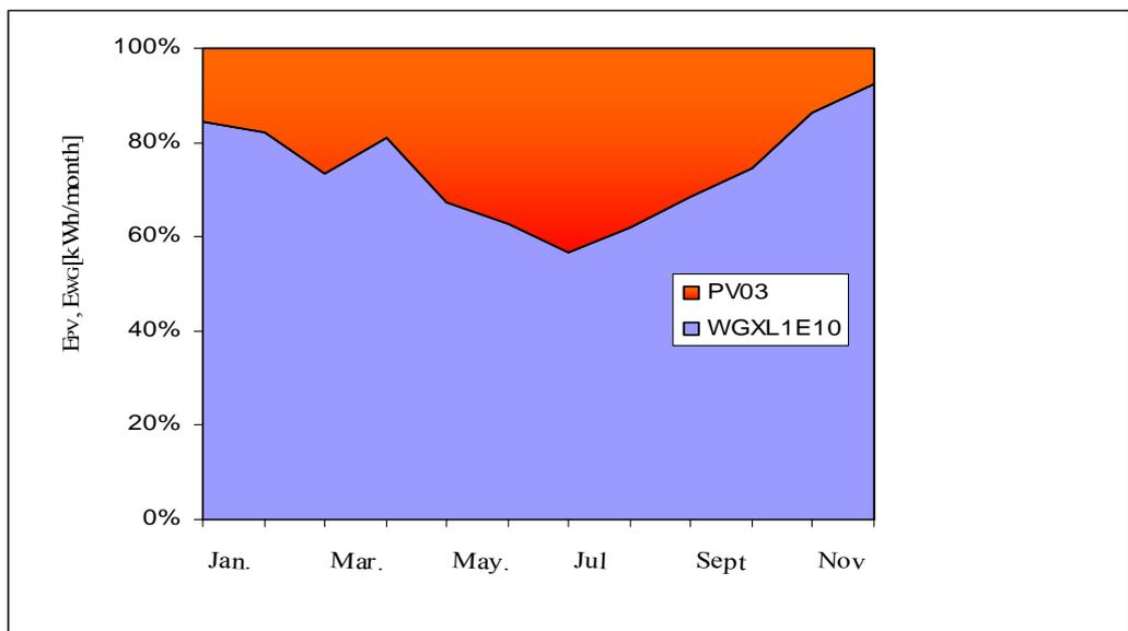
Fig 3.14. The energybalance of 1 kW<sub>p</sub> wind and 0.3kW<sub>p</sub> PV hybrid system
