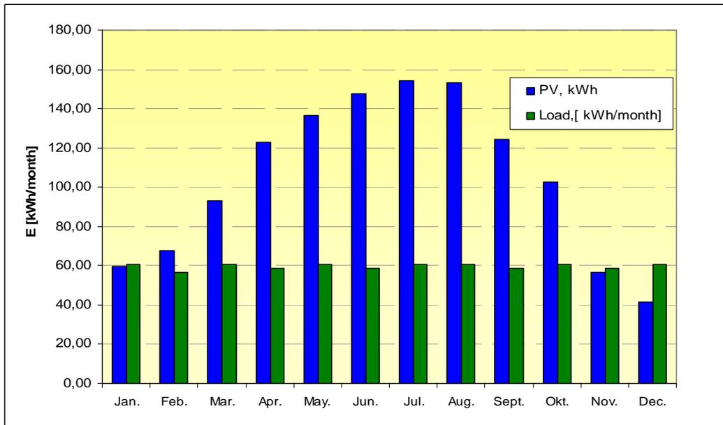
Fig. 3.11. The monthly average energy production of 1 kWp PV system and the monthly load
