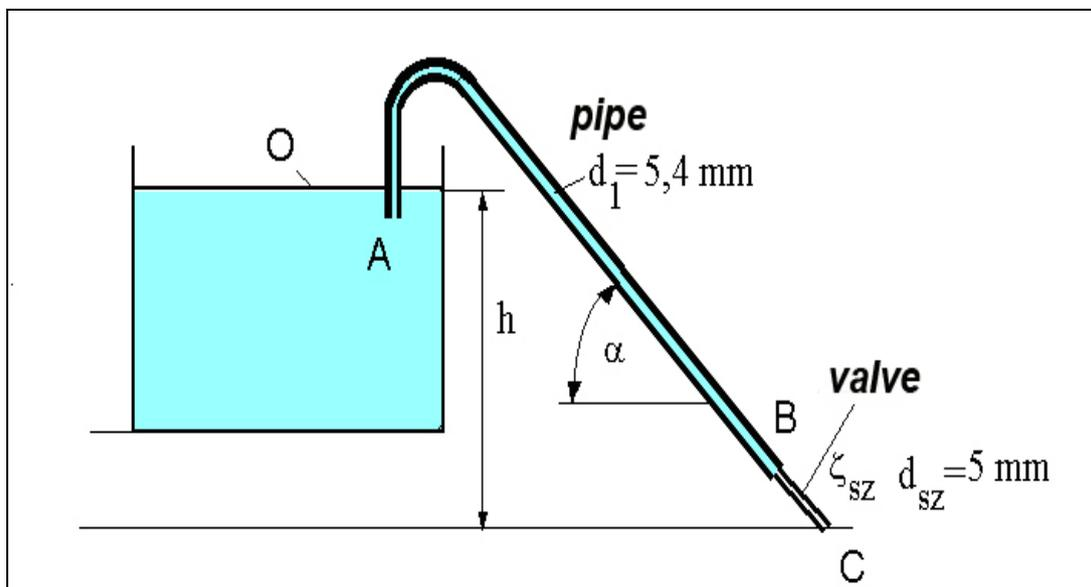
Figure 6: Experimental layout to set different pressures
