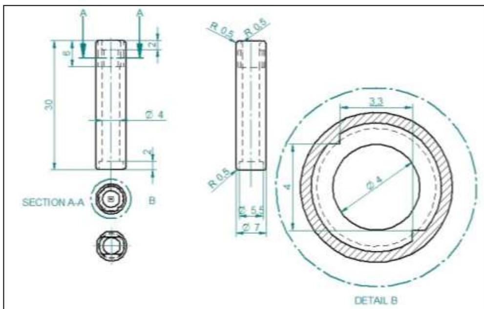
Fig.18. The coupling element
