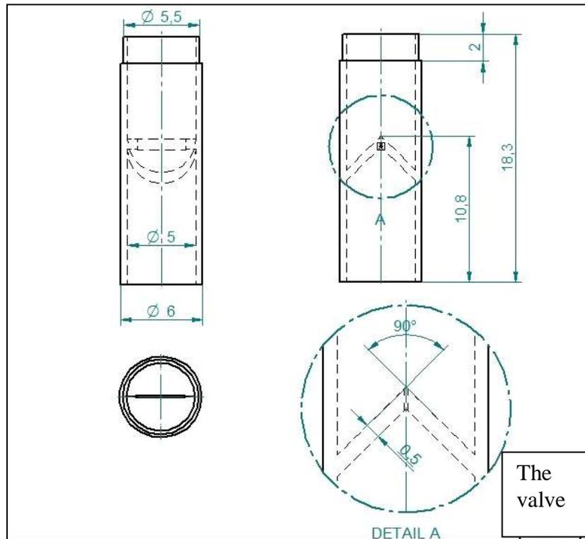
Fig.5. the valve of the short catheter
