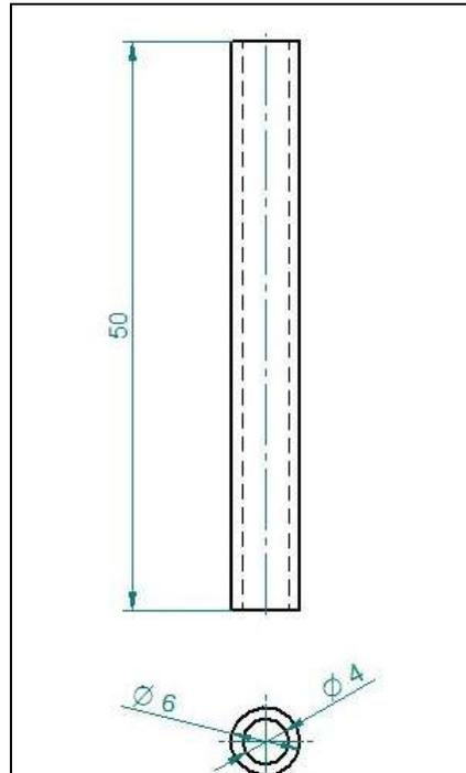
Fig.17. The introducer tube
