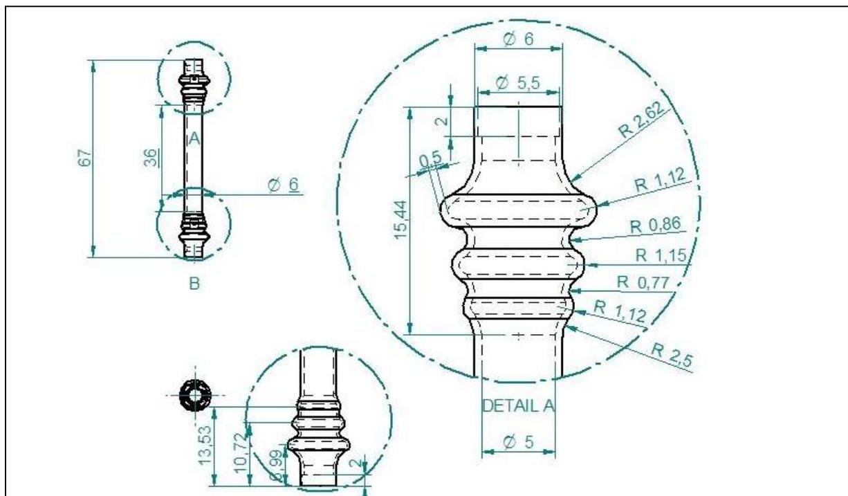
Fig.11. Short catheter- middle stage
