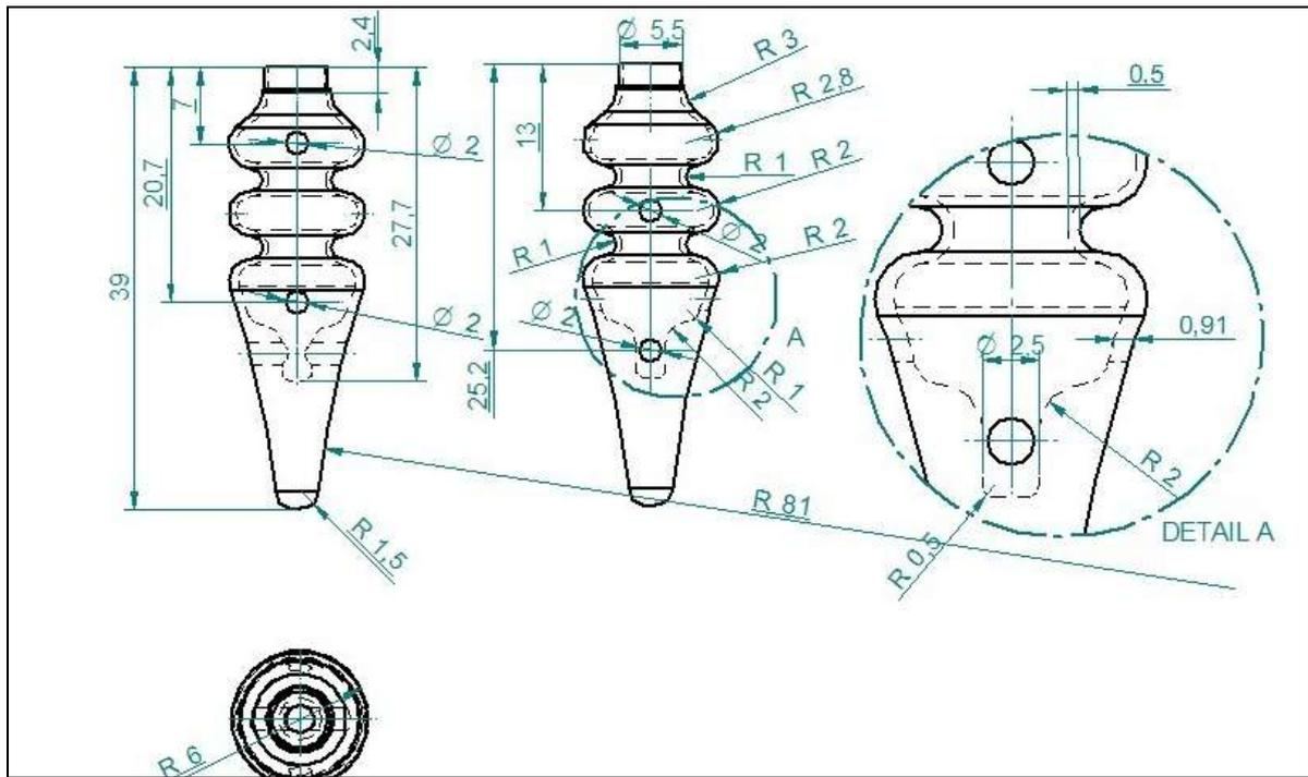
Fig. 12 The tip of the new short catheter
