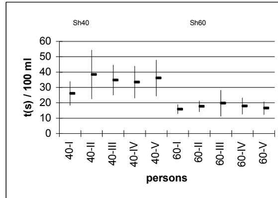
Fig. 21. 100 milliliters water evacuation time, mean and simple deviation in the case of Sh°40 and Sh°60 valves, by five test persons.
