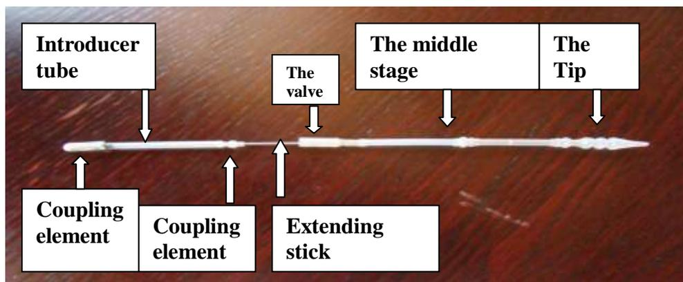
Fig.16. The prototype of the new short catheter
