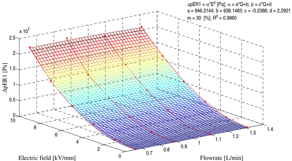
Figure 3.2. Primary pressure increase in the function of the electric field and flowrate (m = 30% additive material concentration TiO<sub>2</sub>/SN150A blend)
