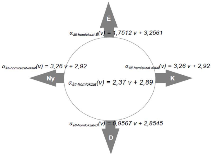
Fig. 5. The averaging of the heat transfer coefficient functions at façade mounted modules
