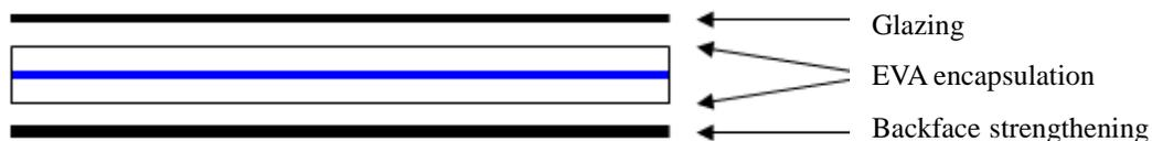
Fig. 3. The structure of a PV module
