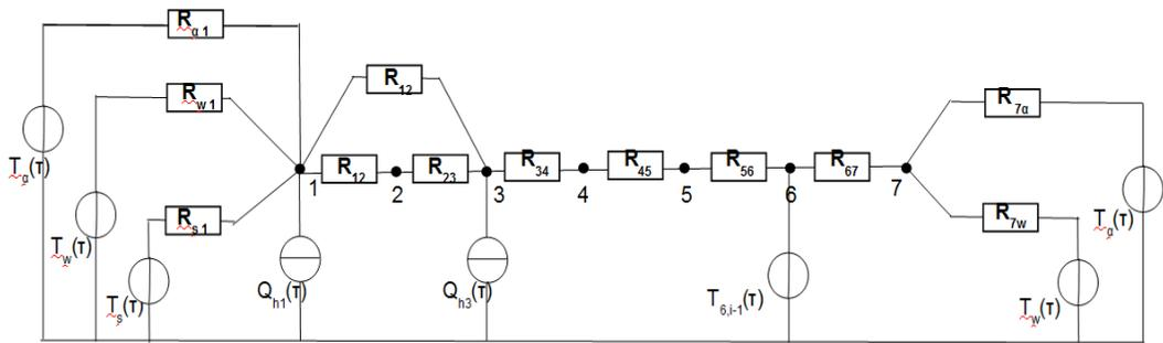
Fig. 9. The heat resistance model of a PV/T module (HR-PVT)
