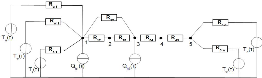
Fig. 6. The heat resistance model of a typical PV module
