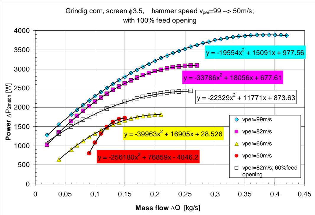
Figure 2.13. Relation of momentary mass flow and power change on shaft to different hammer peripheral speeds in the unsteady state of grinding
