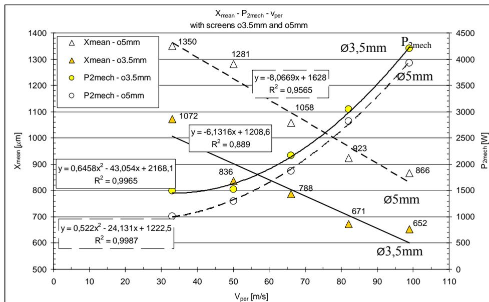
Figure 2.7. The result of increasing hammer peripheral speed on mean particle size  $X_{mean}$  and performance  $P_{2mech}$
