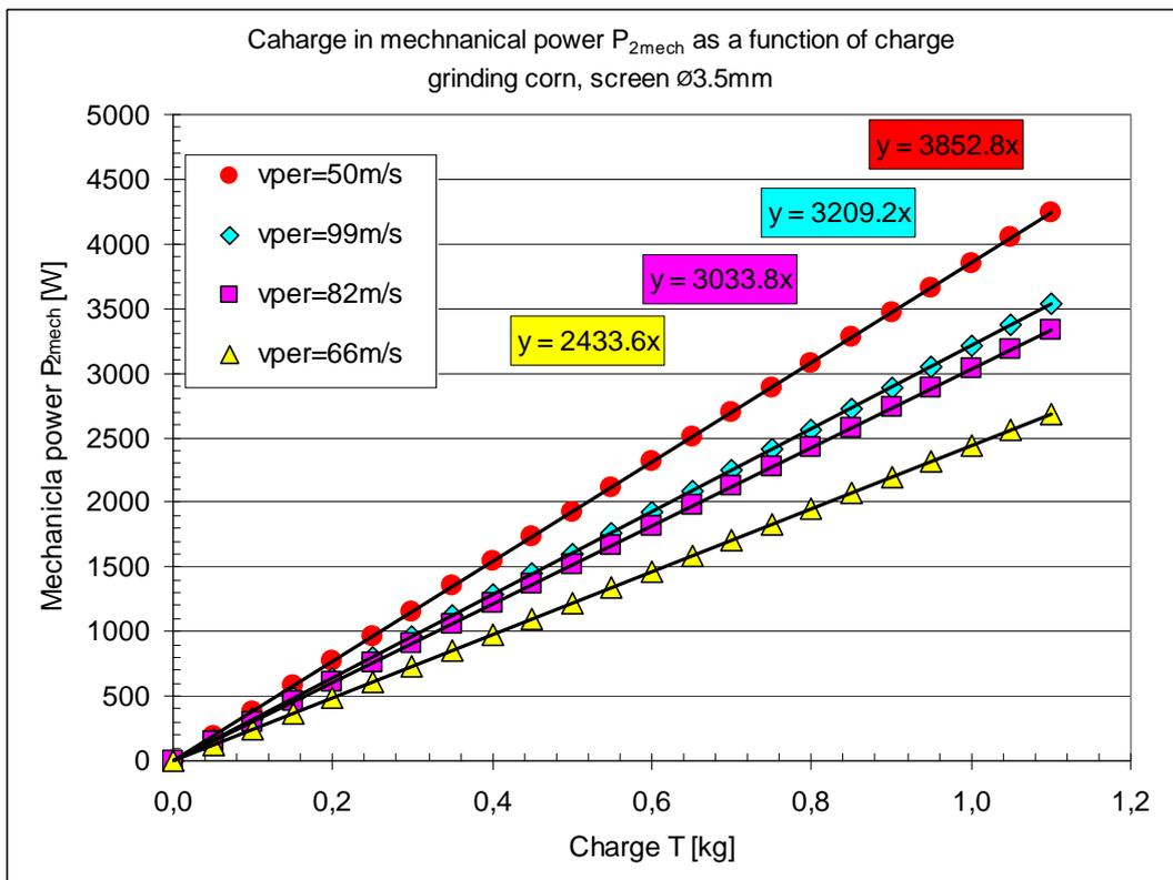
Figure 2.12. Mechanical power as a function of charge in the unsteady phase of grinding
