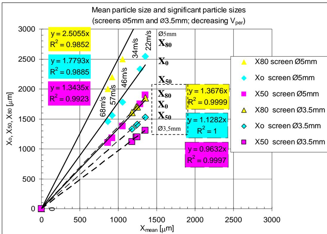
Figure 2.10.  $X_0$ ,  $X_{50}$ ,  $X_{80}$  particle sizes in the function of mean particle size with knowledge of different hammer peripheral speeds
