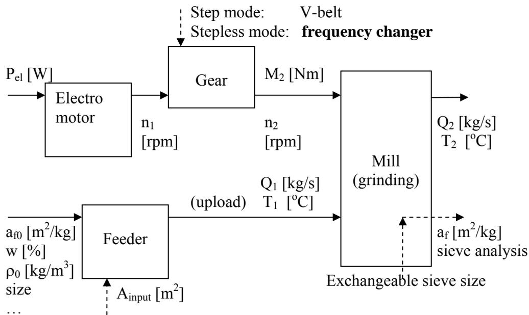
Figure 1.1 The scheme of the experimental apparatus, input, output variables, parameters
