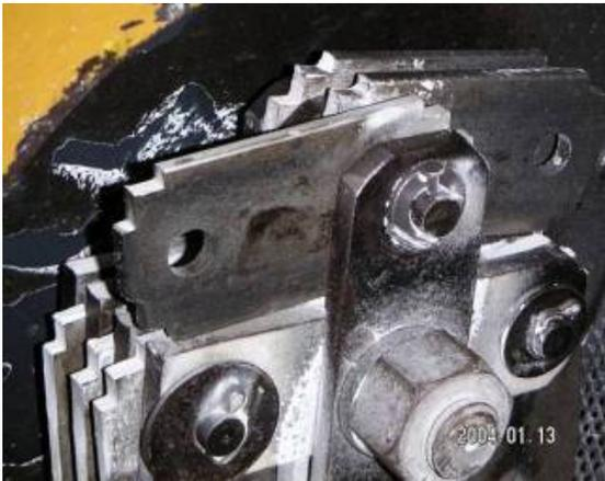
Figure 2.1. Arrangement of hammers in the grinding space
