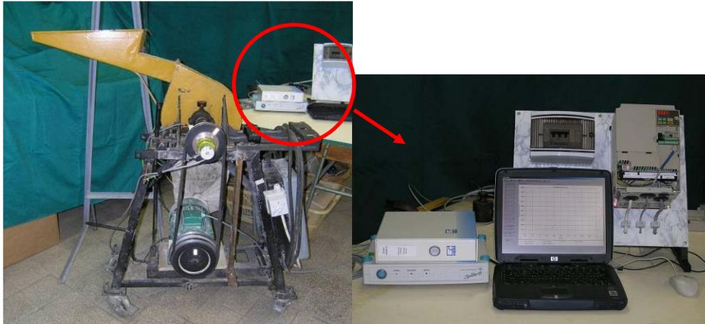
Figure 1.2 Zenit Junior hammer mill – measurement system
