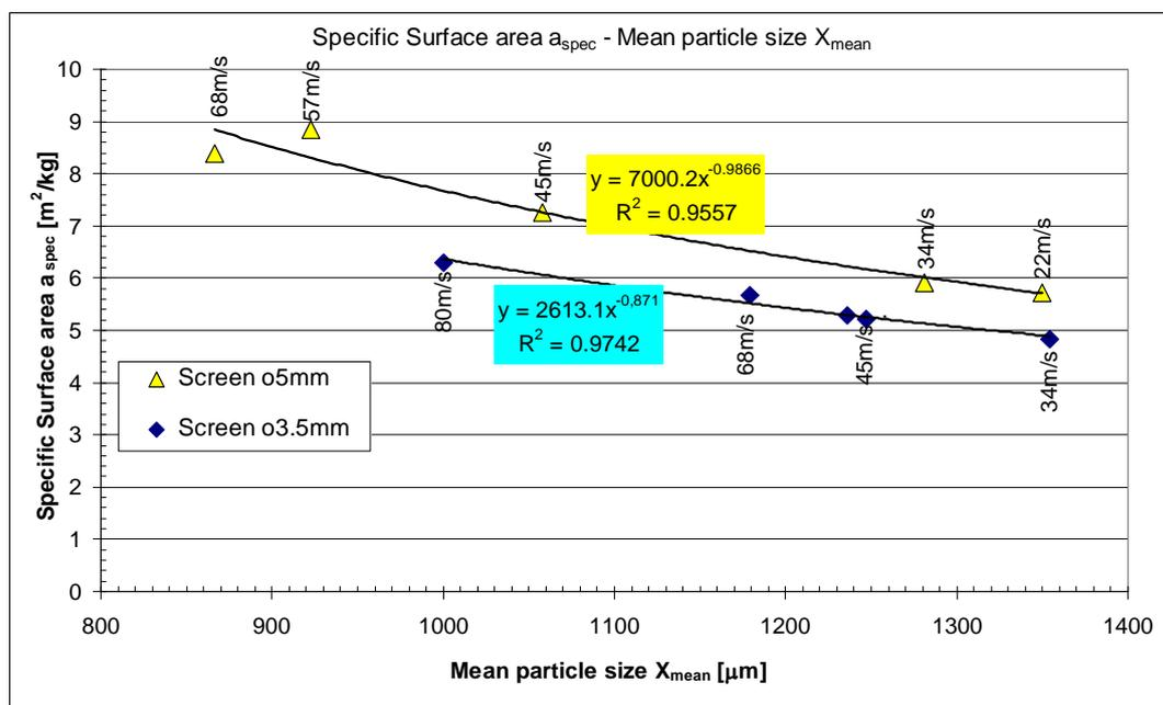
Figure 2.8. Relation between mean grain size ( $X_{mean}$ ) and specific surface, with changing hammer peripheral speed hyperbola
