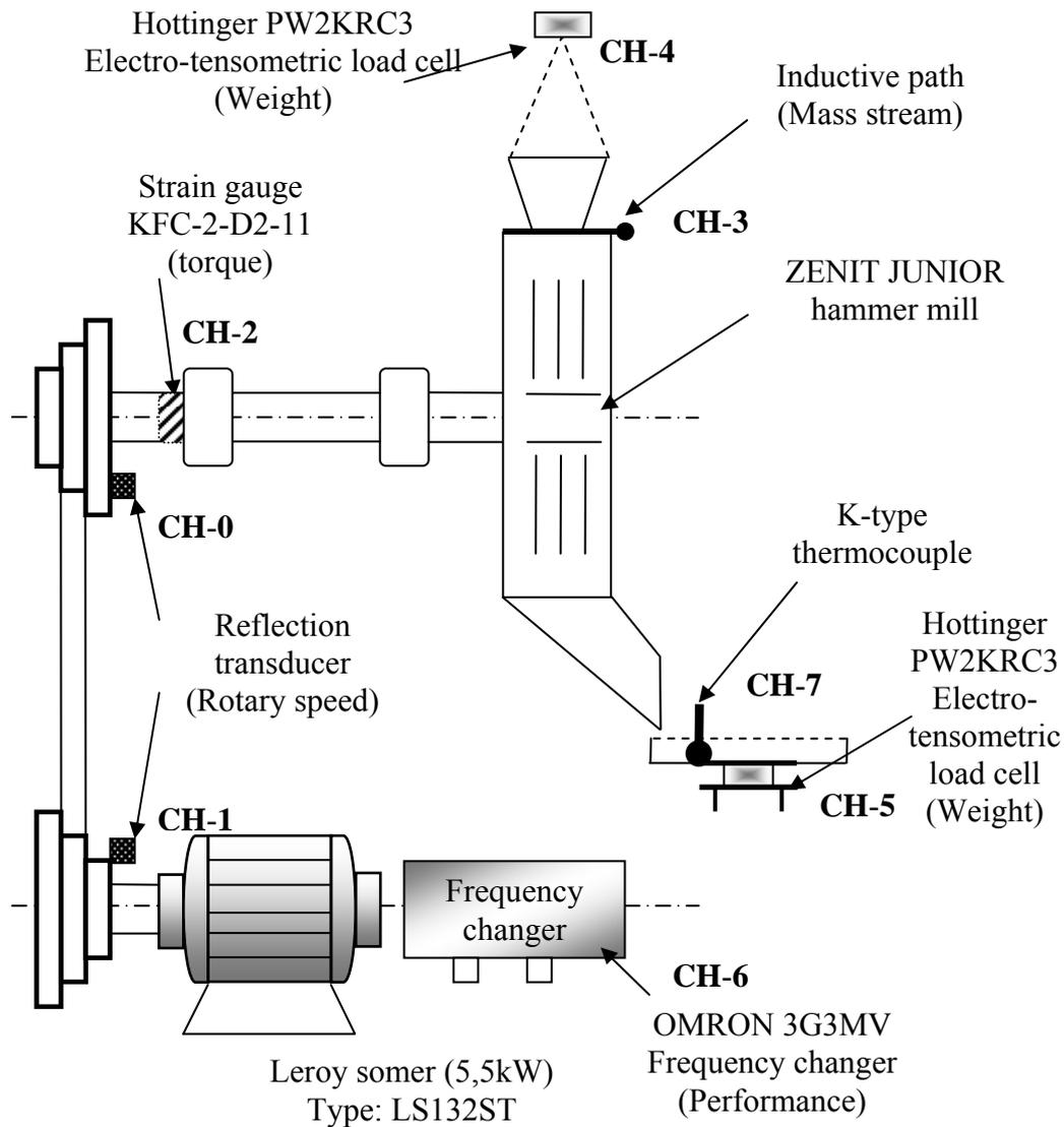
Figure 2.3. The structure of test bench mounted with frequency converter (with measurement point markings)
