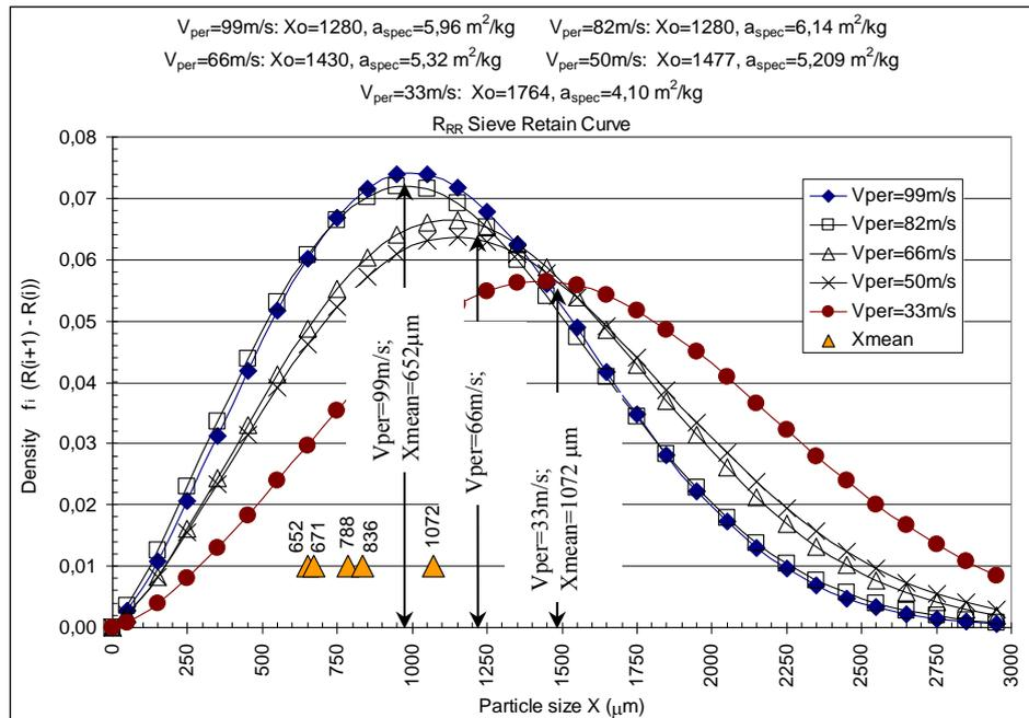
Figure 2.6. Particle size distribution density curve
