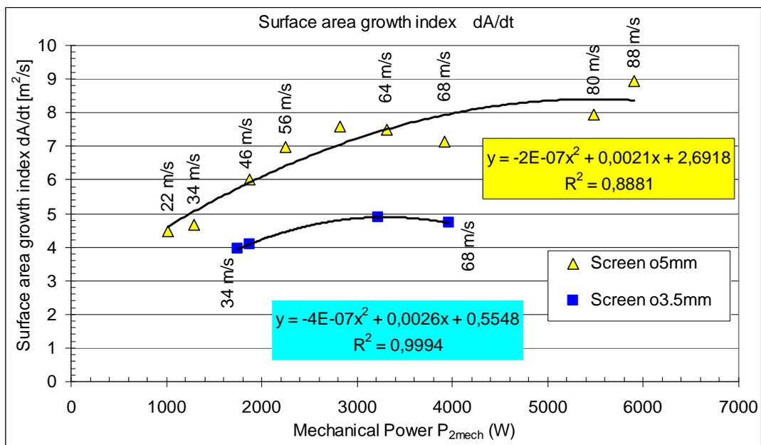
Figure 2.5. Surface growth intensity with increasing hammer peripheral speed is on the second degree in function of performance on shaft
