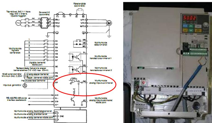
Figure 2.4. OMRON frequency converter and its connection plot
