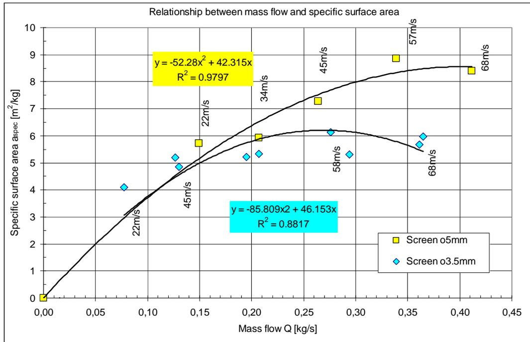
Figure 2.9. The increasing of mass flow with hammer peripheral speed and the formation of specific surface area results in an equation of the second degree
