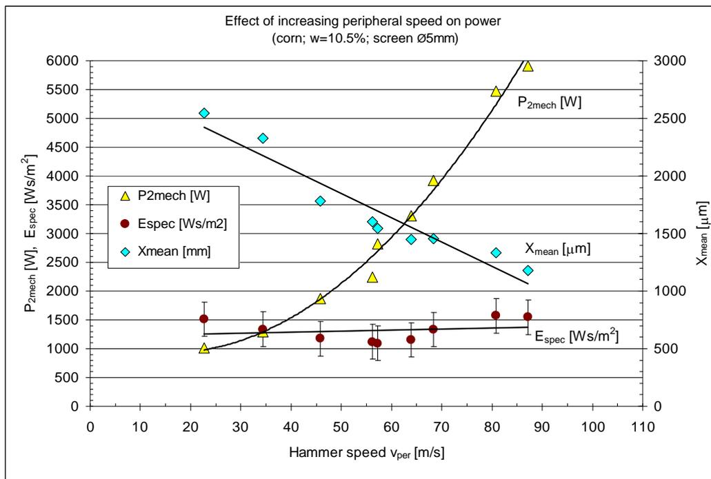
Figure 2.11. Mechanical power ( $P_{2mech}$ ), specific energy requirement ( $E_f$ ) and mean particle size ( $X_{\text{áltag}}$ ) as a function of hammer peripheral speed
