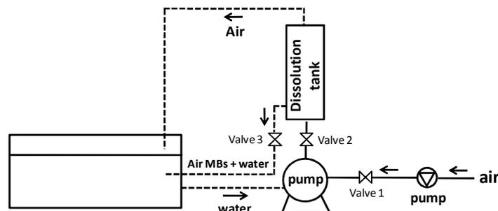
**Figure 4.** Schematic diagram of hot water and microbubbles generation system
