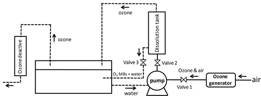
**Figure 3.** Schematic diagram of ozone microbubbles generation system
