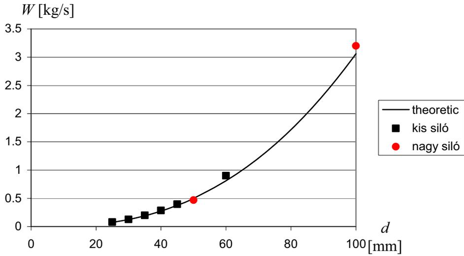
Fig. 11. Measured and predicted discharge rates
