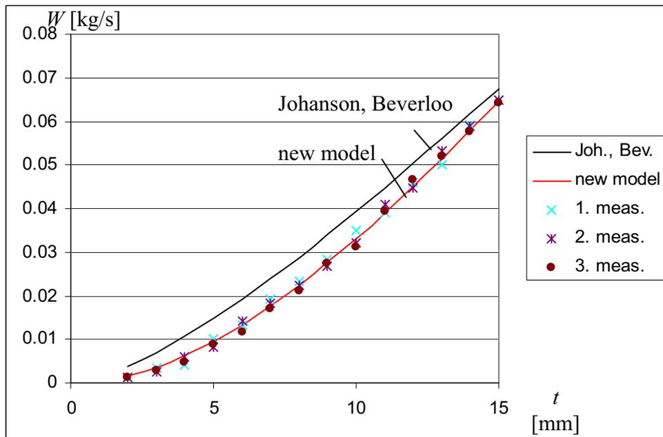
Fig. 9. Discharge rate in function of slot size
