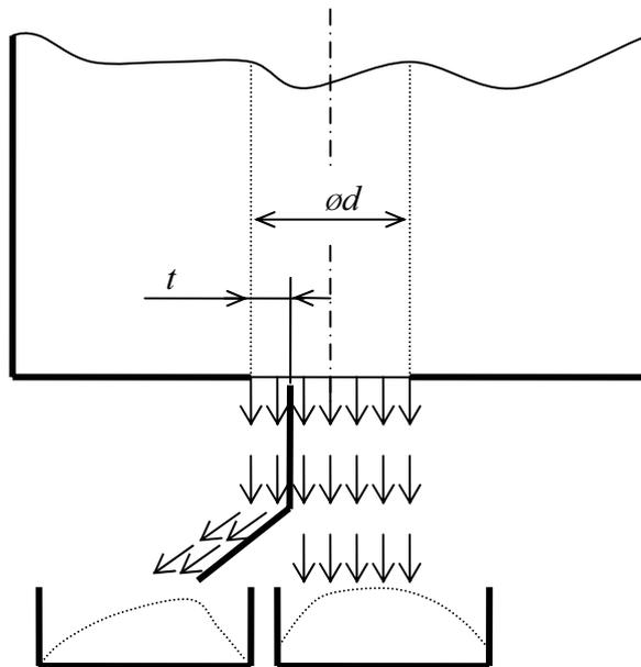
Fig. 7. Measuring of velocity distribution
