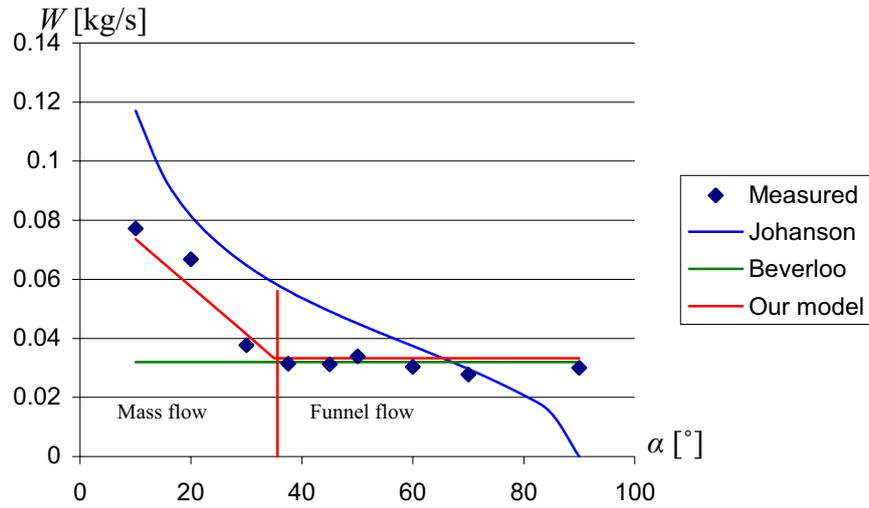
Fig. 13. Measured and predicted discharge rates
