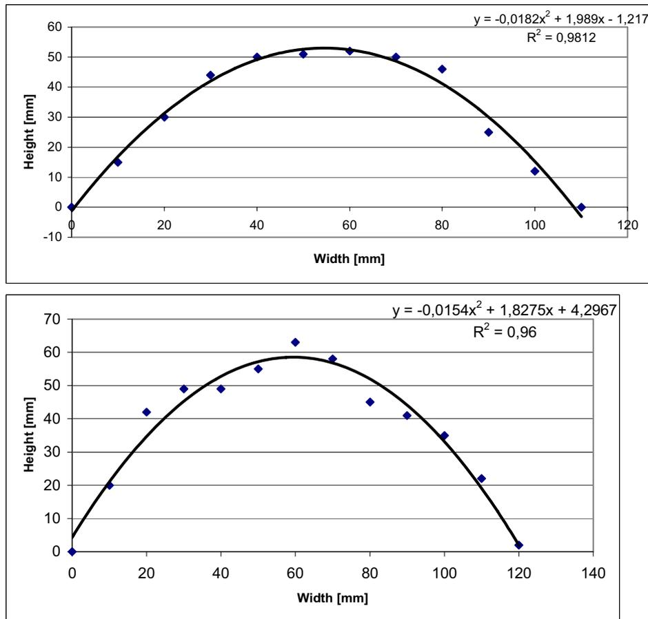
Fig. 4. Measured shapes of arches
