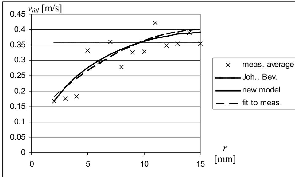
Fig. 10. Velocity in function of outlet radius
