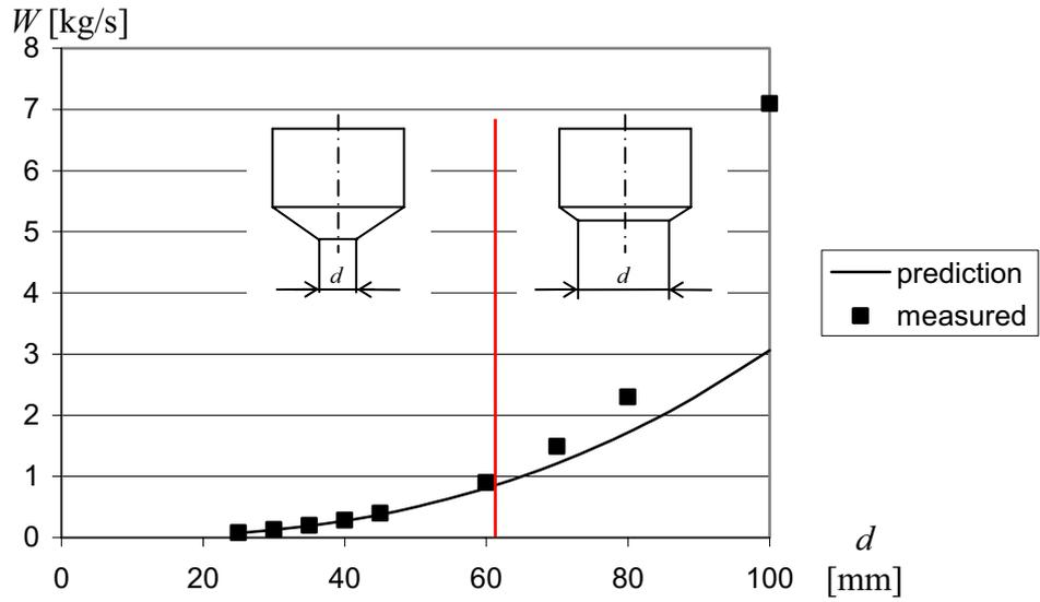
Fig. 12. Measured and predicted discharge rates
