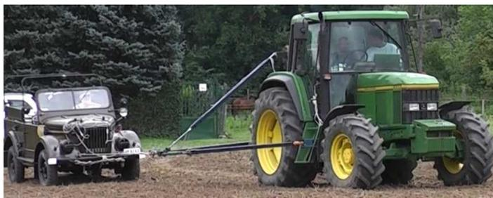
Figure 2.1. Pulling test on arable land: John Deere 6600 and Gaz 69.
