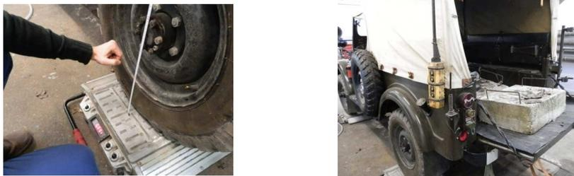
Figure 2.2. Defining the spring stiffness, a) the distance between the center of the wheel and the soil surface, b) extra load on the tire.
