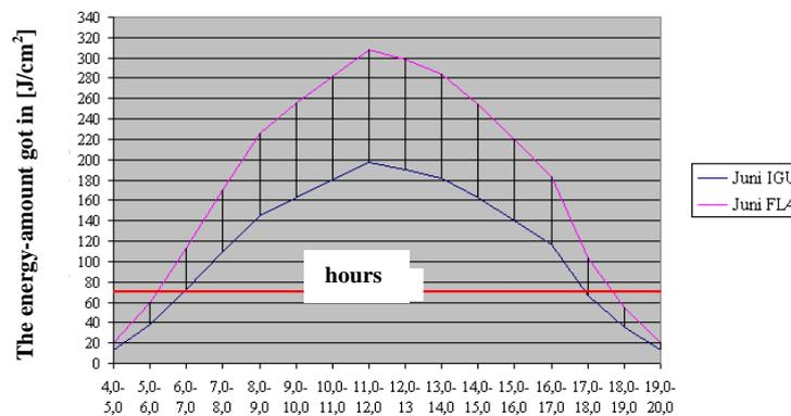
Figure 2. The energy amount got in through the FL4 and IGU glass from the global radiation in June
