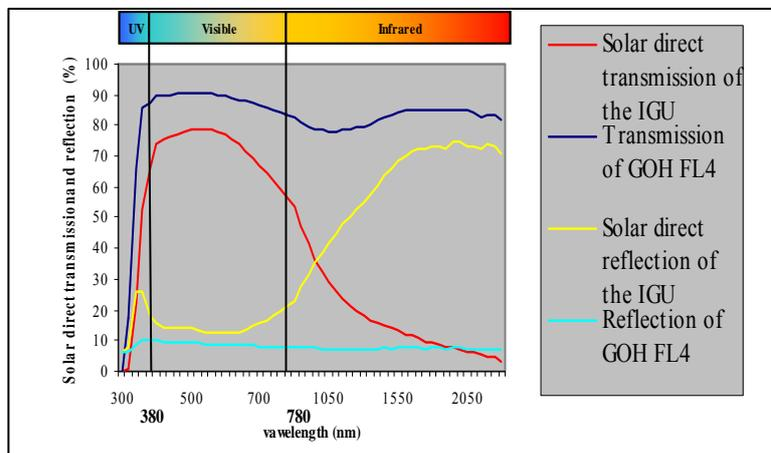
Figure 1. Solar direct transmission and reflection of the IGU and float glass
