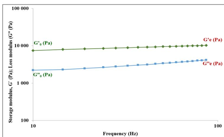
**Figure 2. Frequency sweep rheogram and parameters**
